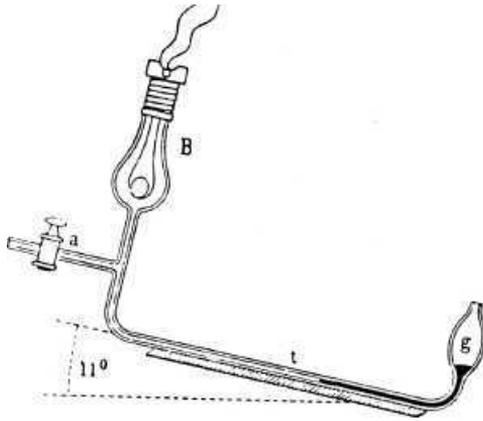
FIG. 26 Electrical air-thermometer. Current in the carbon filament of the bulb B heats air in the capillary tube extension. The capillary tube ends in a small bulb g, filled from a with a solution of alcohol and methylene blue. The temperature is read on the scale t. Bernstein, *Elektrobiologie* (1912) (ref.41).
