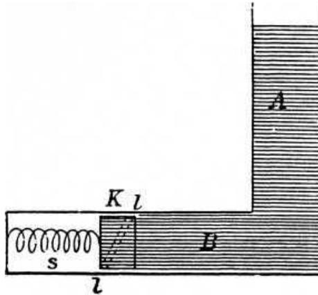
FIG. 17 Pfluger's formal analogy for depicting the principles of nerve and muscle mechanics. The spring  $s$  and piston  $K$  represent the molecular forces opposing the "potential energy" stored in the nerve, represented here by hydrostatic pressure in the tube  $AB$ . Pfluger, *Untersuchung* (1859) (ref. 34).
