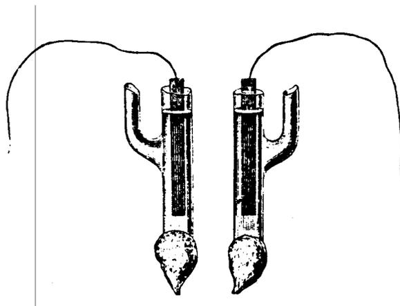
**FIG. 13 DuBois-Reymond's nonpolarizing electrodes.** Zinc strips coated with a layer of zinc sulfate dip into a concentrated solution of zinc sulfate. The tips of the glass tubes containing the electrodes and electrolytes are made of modeling clay soaked in saline solution. Bernstein, *Lehrbuch* (1900) (ref. 40).
