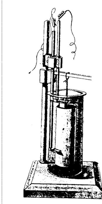
**FIG. 9 DuBois-Reymond's physical model for the muscle current.** A hollow copper cylinder, galvanized on the outside, hangs in a beaker containing an electrolytic fluid. Leads from a galvanometer run to the outside and to the interior of the cylinder. DuBois-Reymond , *UTE, 1* (1848).
