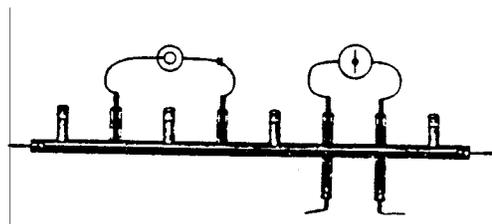
**FIG. 16 Hermann's apparatus for modeling the phenomena of electrotonus.** A silver conducting wire is immersed in a dilute solution of sulfuric acid and placed in a glass tube corked at both ends. Capillary junctions are placed so that recording electrodes and stimulating electrodes can be variously positioned in order to explore effects in both intrapolar regions and extrapolar regions. Biedermann *Elektrophysiologie* (1895) (ref. 39).
