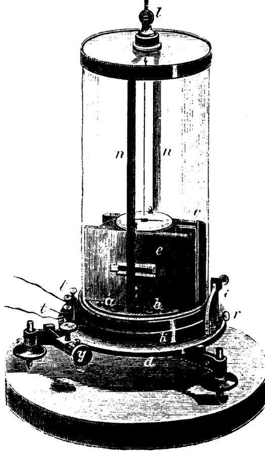
FIG. 2 DuBois-Reymond's multiplier. The conducting wire is coiled some 24,160 times, about the places e. The upper needle is shown suspended by a thread from 1; the lower swings in the plane marked by the slit in e. Current enters the instrument at t. Elie de Cyon, *Atlas zur Methodik der physiologischen Experimente and Vivisectionen* (Grieben, 1876), table xlv.
